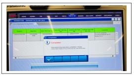
k. Confirm the results then click the ALL DTCs button on the System Select screen to check DTCs.
