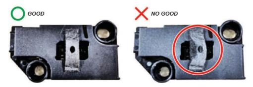
Inspect the microphone assembly using the ANC MICROPHONE CHECK procedure on the next page.
