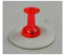
• If the push pin doesn't sit flush or there's resistance, you need to replace the microphone assembly.
