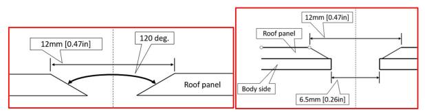
• Treat the cut remaining shaft of the rivet so it does not protrude above the rivet head. See images below.
