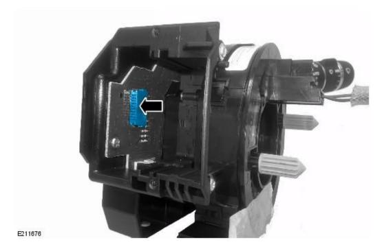
With the lighting control switch removed, apply the Nyogel to the electrical contacts surface.
