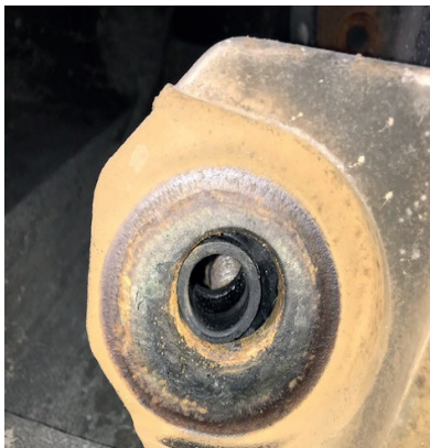
Figure 6 - Bushing Incorrect Fit in the Axle
