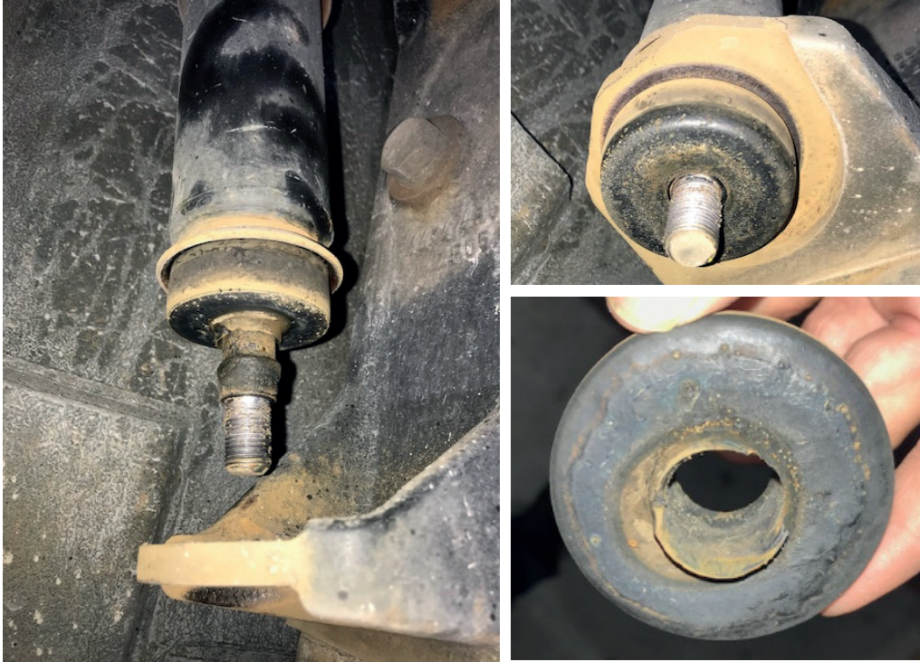
Figure 5 - Wear Marks on Axle
