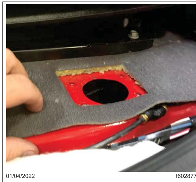
Fig. 21, Trimmed Cab Floor Mat
