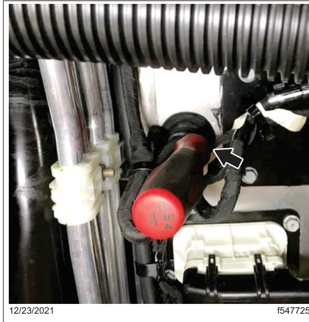
Fig. 13, Screwdriver Inserted to Assist with Passing Through the Cable Tie
