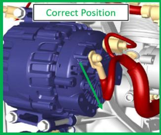
• If the connection is routed correctly (as shown), no further work is required.
