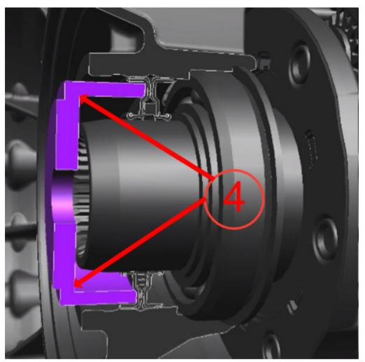
One tip for installation is to determine case design level, and put a mark on the outside of J-45228 at 17 mm for first design and 19.5 for second design (3) as a visual aid to stop when the mark is even with the case.
