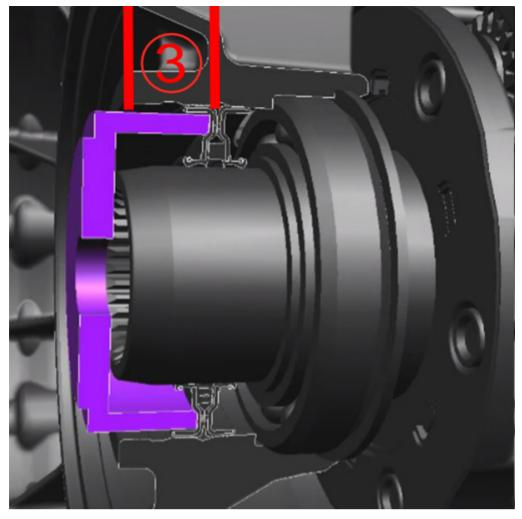
To verify correct installed depth using a vernier caliper check the distance between the case and the outer part of the seal.
