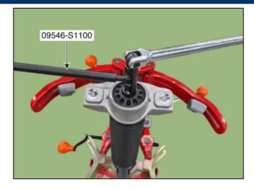
8. Remove the insulator assembly (G) and install the new insulator part.
