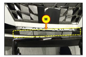
13. Remove both front bumper side moldings (L).
