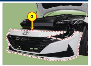
8. Place the front bumper face down for access to the bumper moldings.
