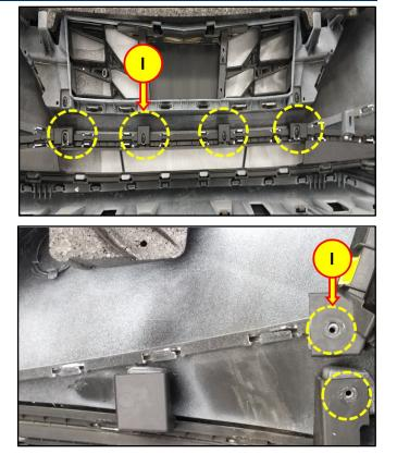
11. Using cutting pliers, cut off the locking tabs (J) on the side moldings and lower molding.
