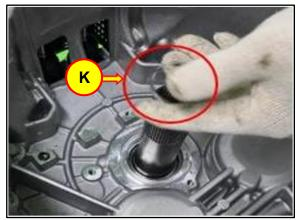
16. Check the marked size of the snap ring and prepare a new snap ring two increments lower in size.
