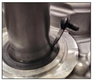
9. Reassemble the hook to the puller assembly and adjust the lever stand-off to rest on the transmission case.
