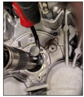
11. Use snap ring pliers (H) to open the snap ring enough to get a small flat blade screwdriver between the shaft and snap ring.
