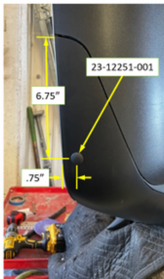
Figure 1: Installation of push pin - screw.
