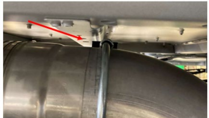
Figure 3. Exhaust Bracket reinstalled and Exhaust Clamp loose.
