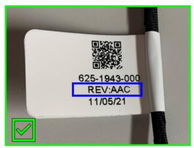
**4.** If the **INCORRECT** harness is installed, the HomeLink Function will not operate. The mirror icons located above the HomeLink buttons will not illuminate. **ALWAYS** confirm the icons illuminate after installing the Auto-Dimming HomeLink Mirror accessory.
