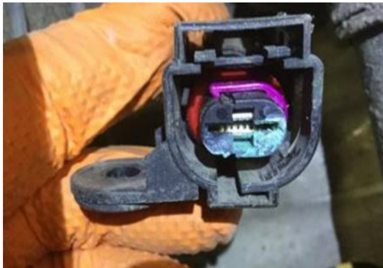
Figure 4: Oxidized connector at T1c
