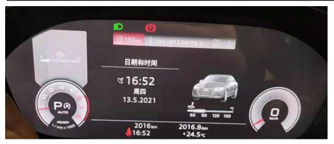
Figure 1-4: example pictures of white sheen on the Audi virtual cockpit
