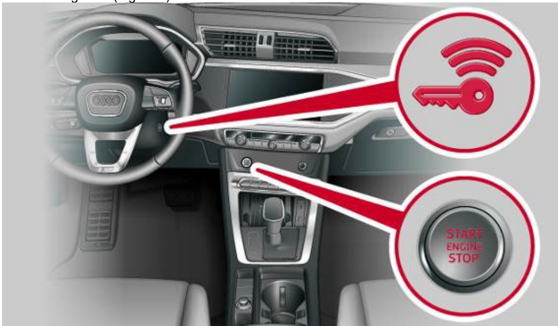
Figure 2. Key reader coil location.
