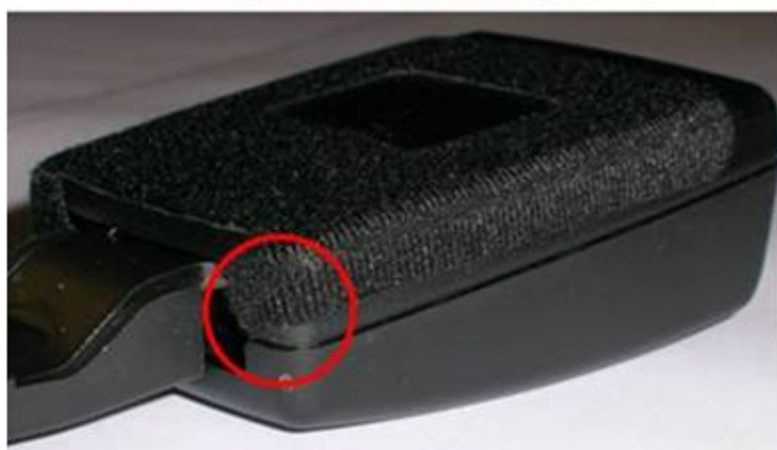
Figure 1. Felt mat 8V0 858 541 attached to belt buckle.
