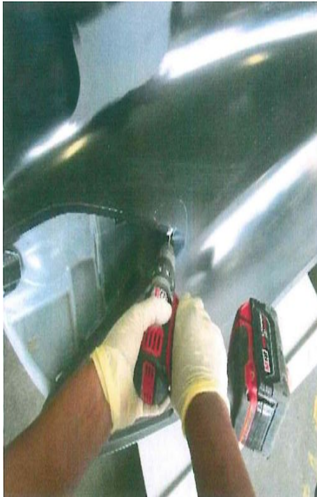
Drill hole at end of crack
