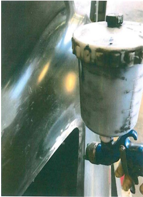
Spray primer on repaired area
