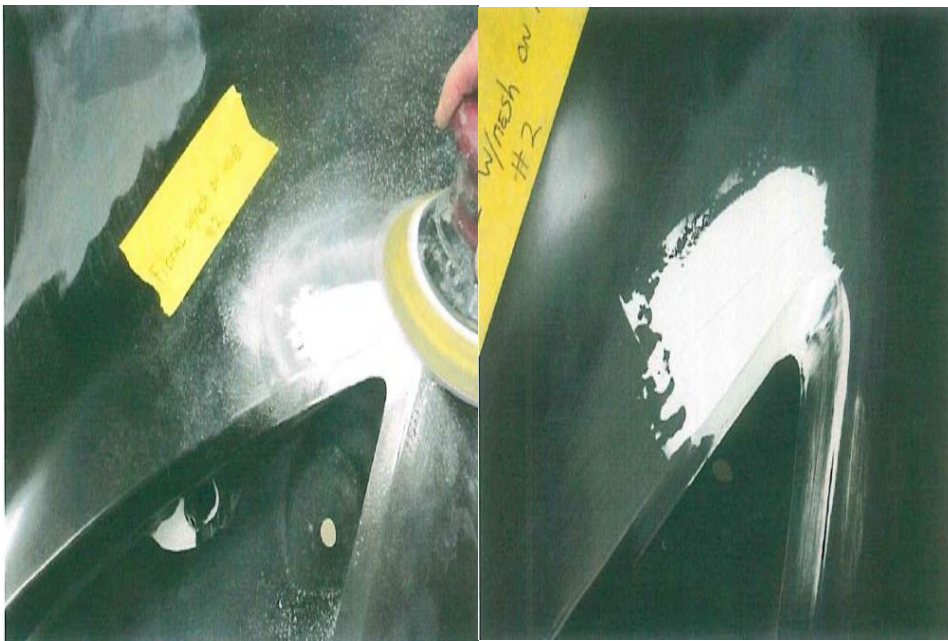
Sand metal glaze with 180 grit sand paper
