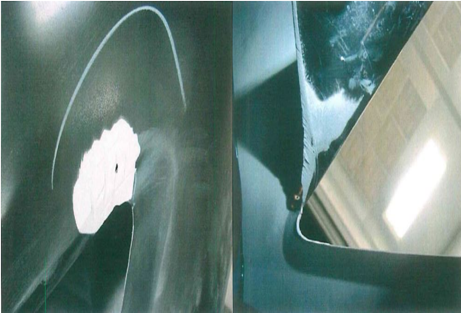
Grind the topside at least 1 inch by 2 inches ( depending on the crack size )
