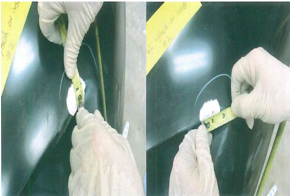
Measure the crack
