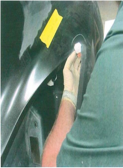
Put tape upside down and layer Fibral and mesh on sticky side of tape so it will stick to under side of hood
