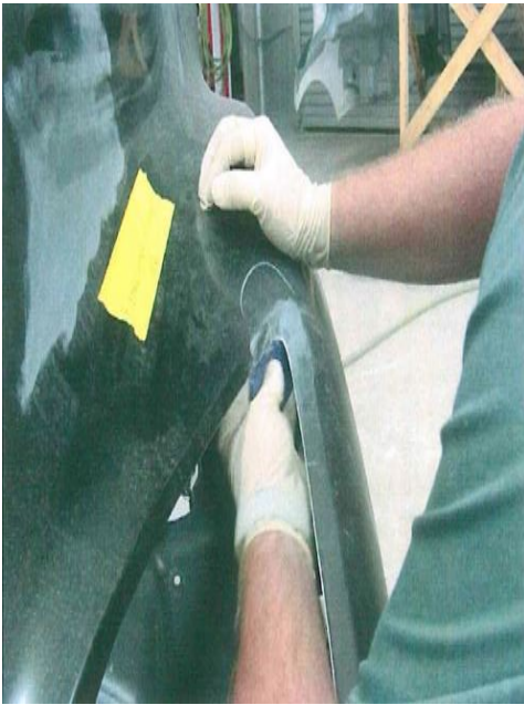
Sand crack area with 80 grit
