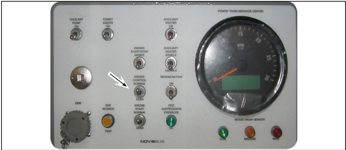
Figure 2 - Engine Control Box
