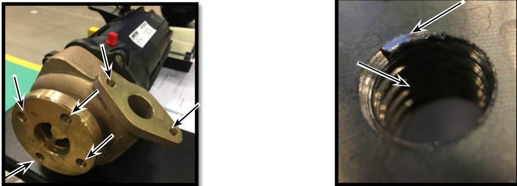
Figure 18 - Inspect the Threaded Holes for the Presence of Burr
