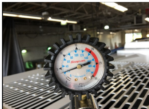
Figure 11 - Pump the Pressure Up to 20 to 21 PSI
