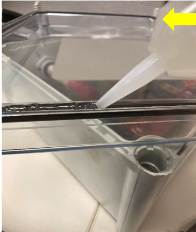
Figure 6: Application of NyoGel on Cover Seal
