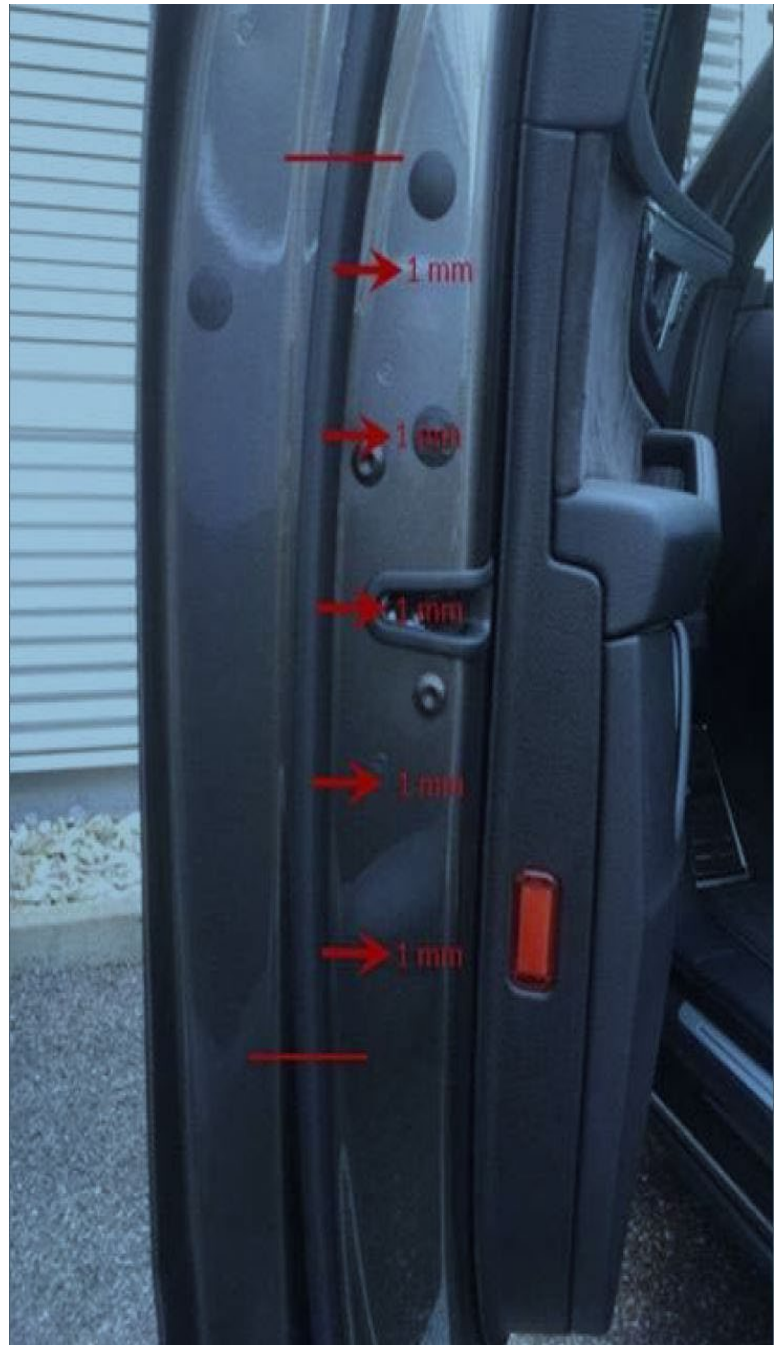
Figure 3. Install the new outer door seal with an inward offset of 1.0 mm.
