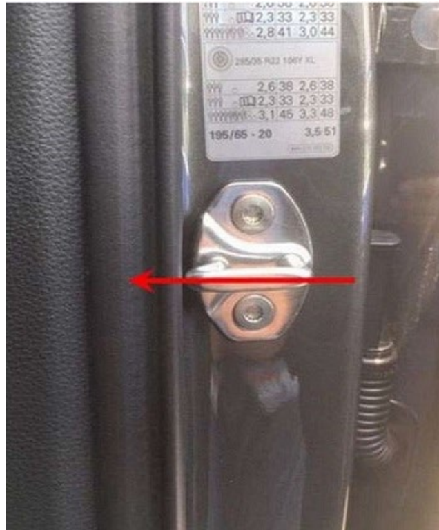
Figure 1. Adjust door striker inward by at least 0.5 mm.
