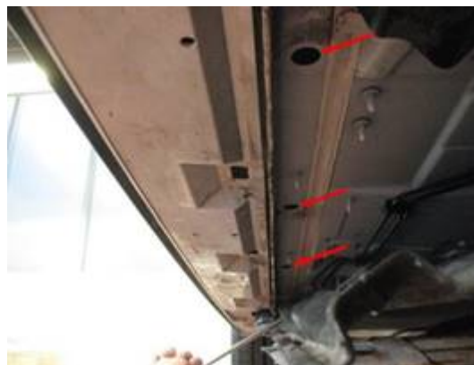
Figure 1. Access to the side member plugs.
