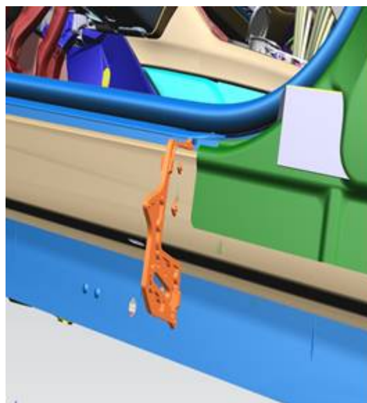
Figure 6. Side member cavity sound absorber.
