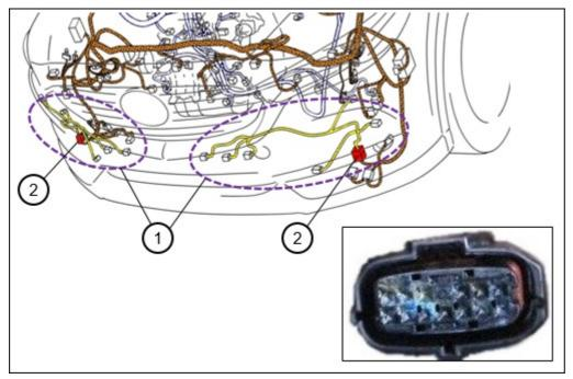
To eliminate this concern, the production process of the front harness short cord has been improved to increase waterproof performance.
