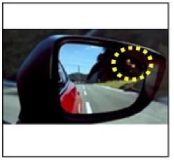
Due to BSM control module production variances, a false detection may occur in some units when the BSM temperature in the control module has not yet reached normal operating temperature. To eliminate this concern, the control logic of the BSM control module has been modified.
