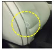
This is caused by the piping of the front seat back trim rubbing against clothes when passengers get in and out of the vehicle, fraying the seam, and resulting in protrusion of the plastic core wire.
