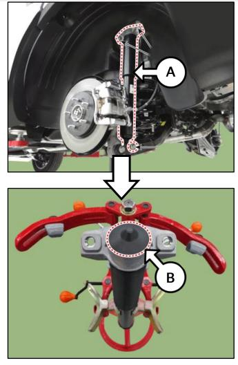
Reinstall the reassembled rear shock absorber
