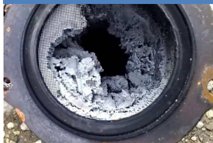
Eroded and broken Catalyst
