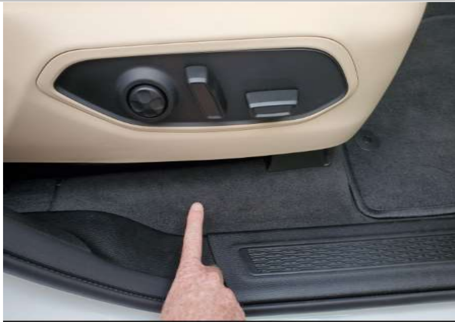
Location just in front of B-pillar near front door sill at area where the B-Pillar HVAC Duct Clips Over
