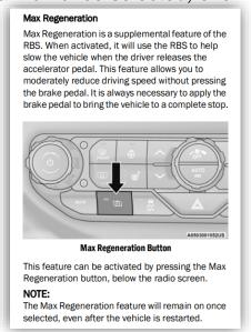
**Repair:** A Software concern is causing the Max Regeneration feature not to remain on after restarting the vehicle. Part replacement WILL NOT correct this concern. A TSB software package which will update multiple modules has an estimated release date within the 3<sup>rd</sup> quarter of 2021. This SOL will be deleted once a resolution is released to the field.
