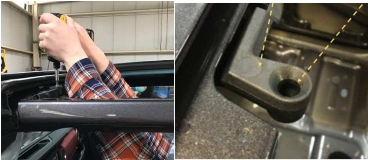
Fig. 6 Drilling Hole From The Top
