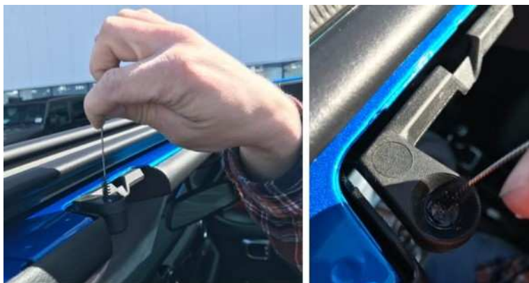
Fig. 7 Applying NLGI Grade 2 White Silicone Grease
