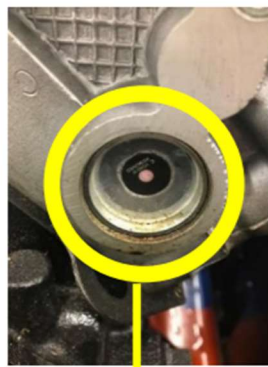
Overheated Pink Sensor 255°F Coolant Temp
