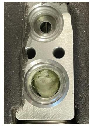
The possible affected vehicle dates are from 9/9/2020 to 9/24/2020. If the vehicle falls in this build date range the SOL should be performed if any restriction is found. If you have a vehicle that you feel is outside of these dates and exhibits debris as shown above a STAR case should be created for further assistance.
