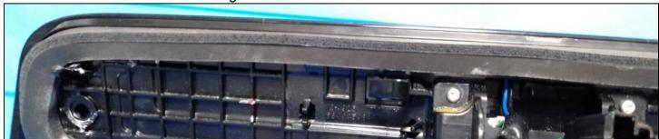
Check: once the CHSML is installed onto the vehicle there should be no gasket visible from the top or the sides.
