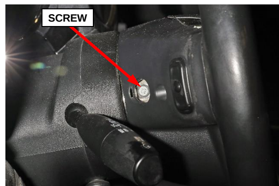
Figure 2 – DAB and Floating Horn Switch Unit Screw
