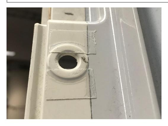
6. Reinstall the 2 T-nut screws per side, torque to 14 Nm.
