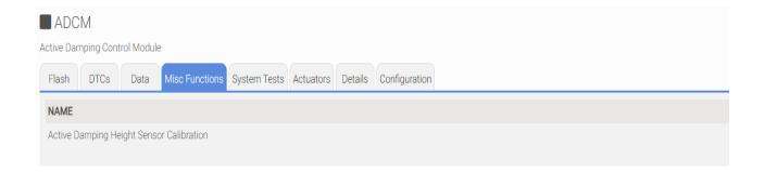
NOTE: All doors must be closed during calibration and vehicle must be on the ground.
