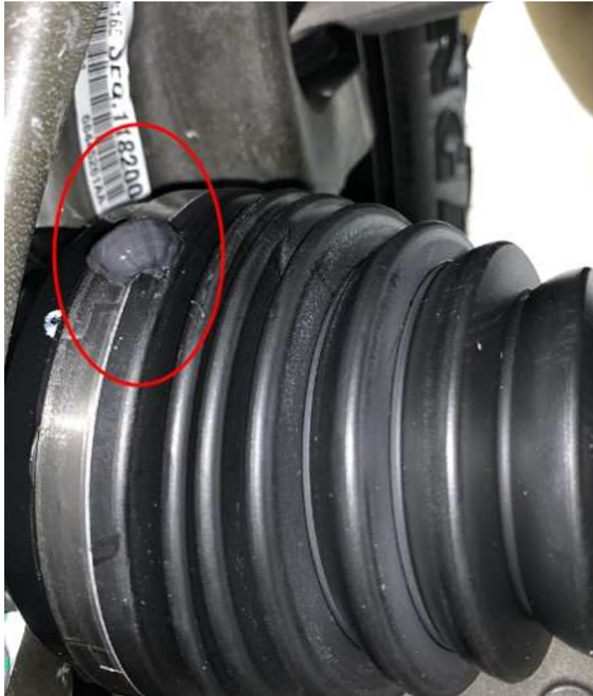
Fig. 5 Boot Grease Leak
