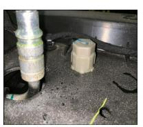
Use Leak Detector Sniffer in This Area as Shown Below.
