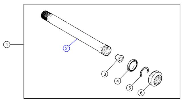
Replace as entire kit (#1) - Intermediate Shaft Kit. Replace axle outer shaft also
