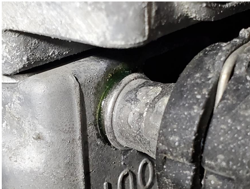
Green Assembly Lubricant On PPU Coolant Fitting
