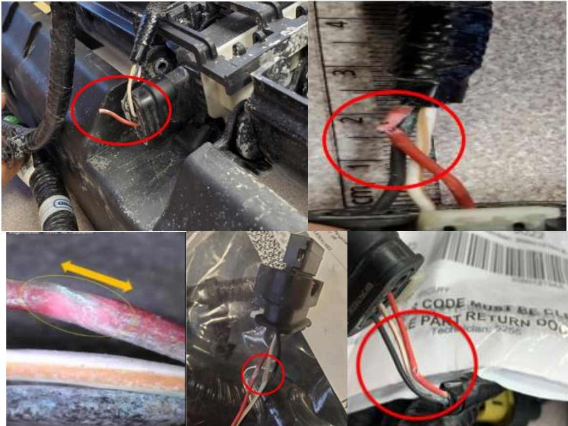
Damaged AGS Wiring Harness Near D2826A
