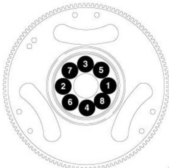
Fig. 4 Flex Plate Bolt Sequence
