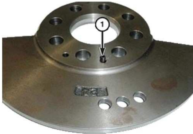
Fig. 3 Counter Weight Dowel Pin Location
