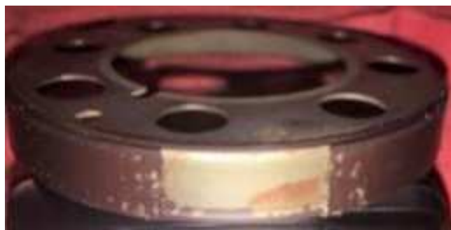
Fig. 1 Missing Magnetic Material On Tone Wheel
