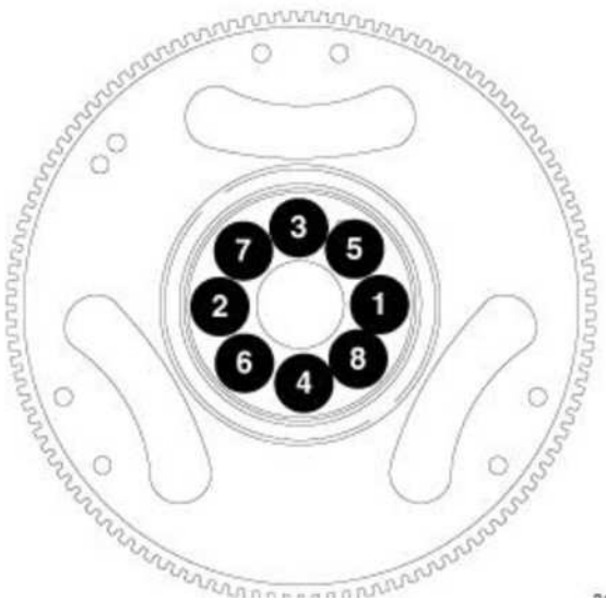
Fig. 4 Flex Plate Bolt Sequence
