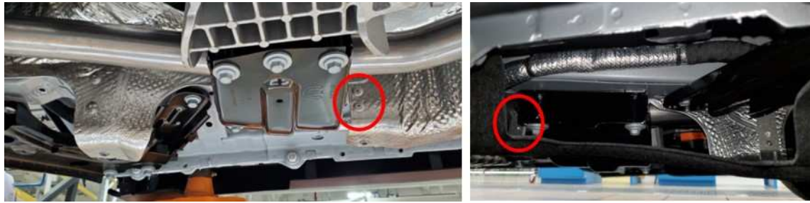
Fig. 1 Front Right Heat Shield Rivets
