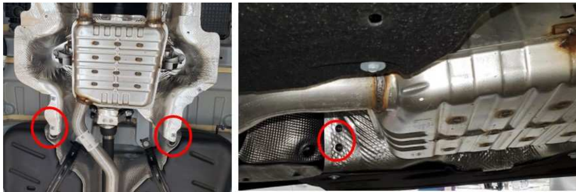
Fig. 3 Mid Heat Shield Rivets
