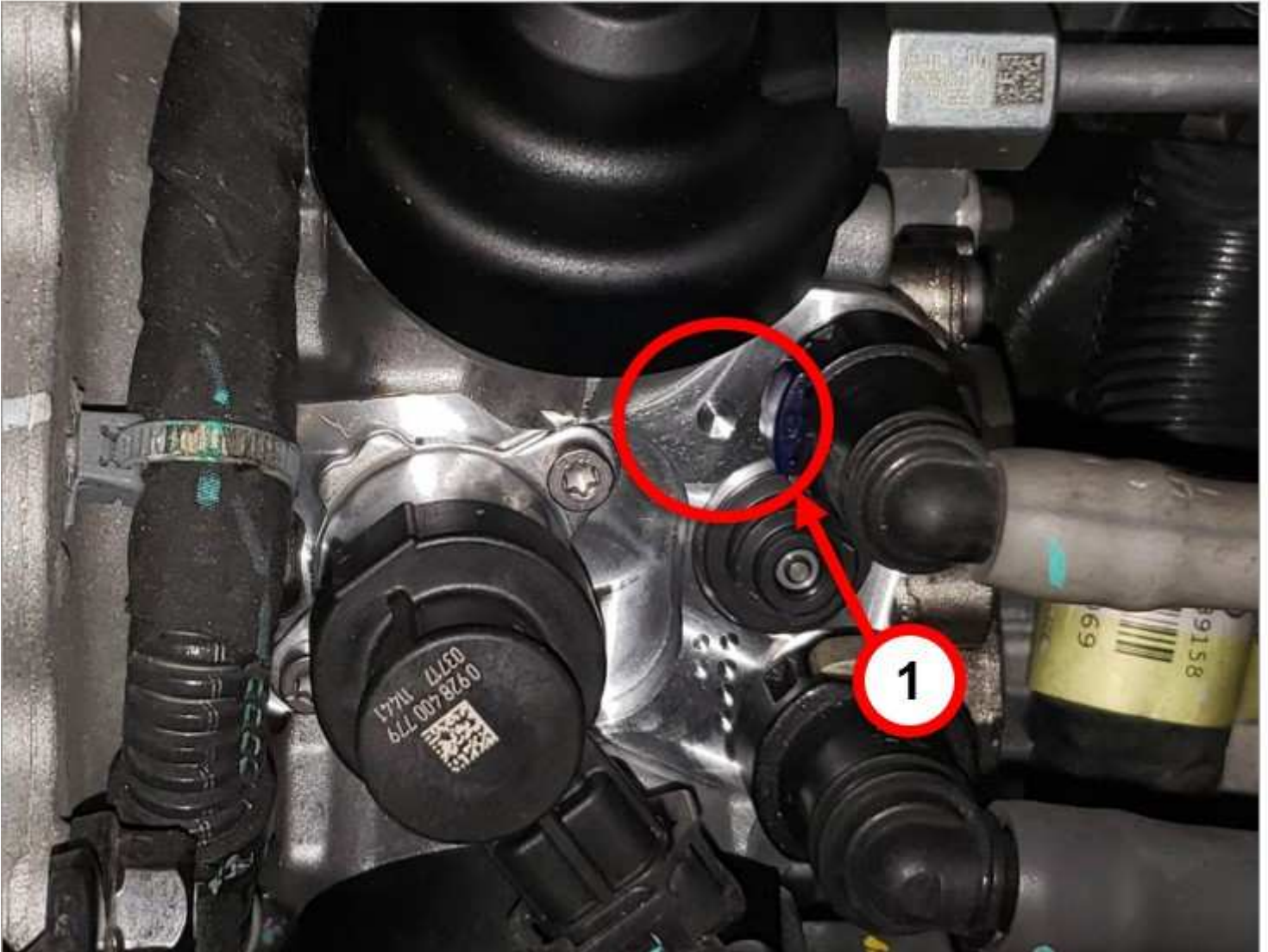
Fig. 1 New Style Symmetrical Cam Design Pump
