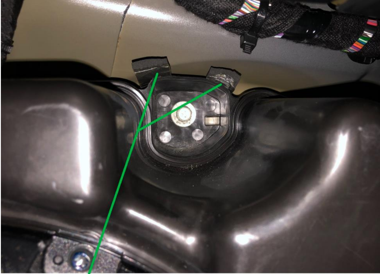
FOAM TAPE INSTALLED TO ELIMINATE BSR
