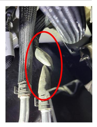
As seen above. The abrasion resistance sleeving may need to be pushed back and away to expose the kink.
