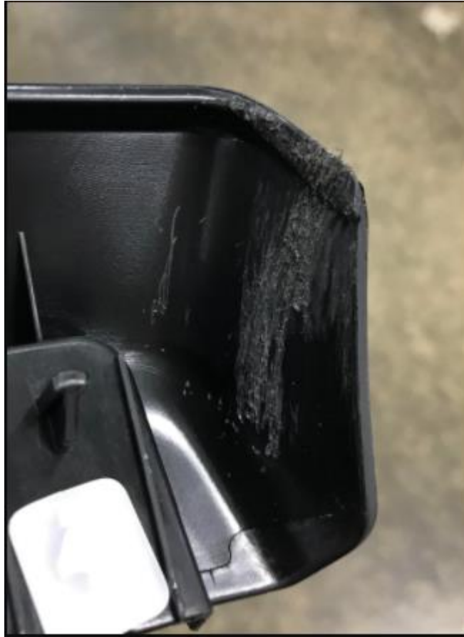
Figure 3. Wheel Spat inside surface filed down
